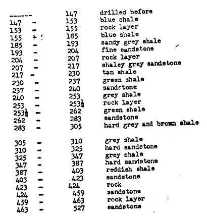
water level 180 feet bailed 10 gallons per minute at 190 feet well cased with 4 inch 11 pound casing
